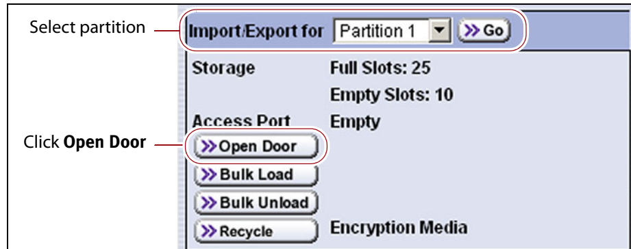
Figure 317 Select the partition and then click Open Door to open the access port.
