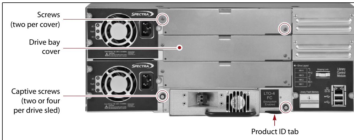
Figure 16 Loosen the captive screws securing the drive bay cover to the library.
