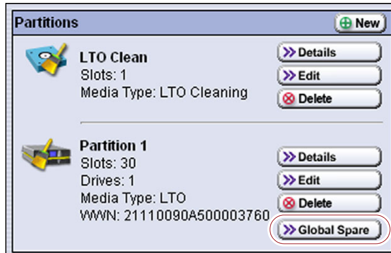
Figure 282 Click Global Spare to begin the process of replacing a partition drive with a Global Spare drive.
