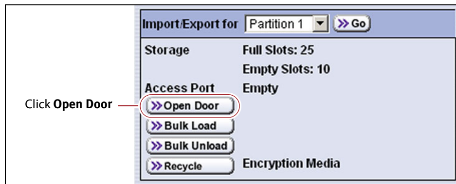
Figure 156 Click Open Door to open the access port and remove the cartridge.
