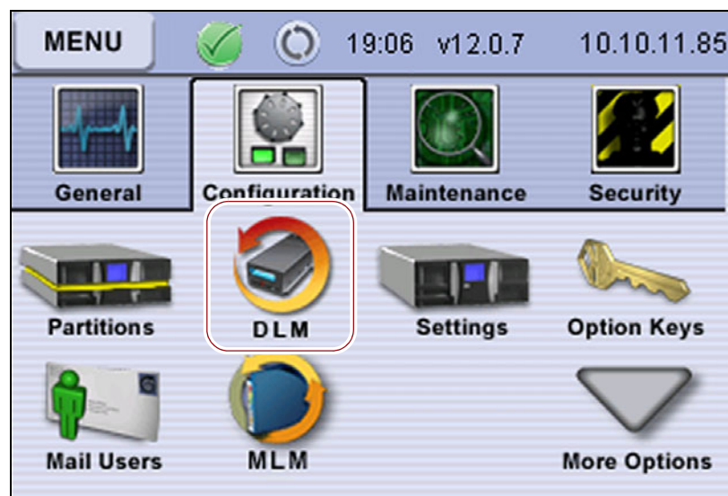
Figure 185 Enabling DLM changes the Drive icon to a DLM icon in the Configuration menu.
