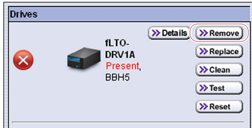
Figure 327 Click Remove next to the drive you want to permanently remove from the library.
